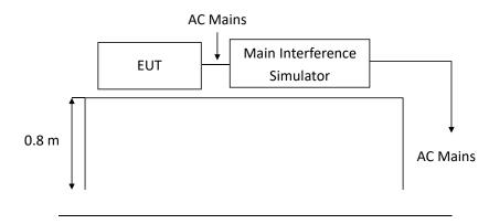
Remark: Combination wave generator and decoupling network are included in test generator.
